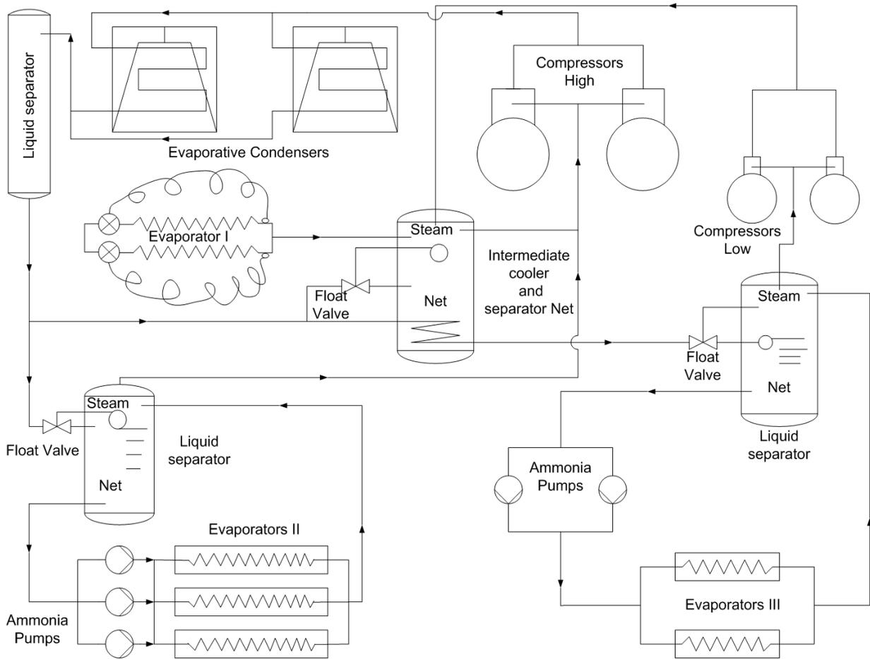
Fig. 3. Vapor-compression cooling system [13].
