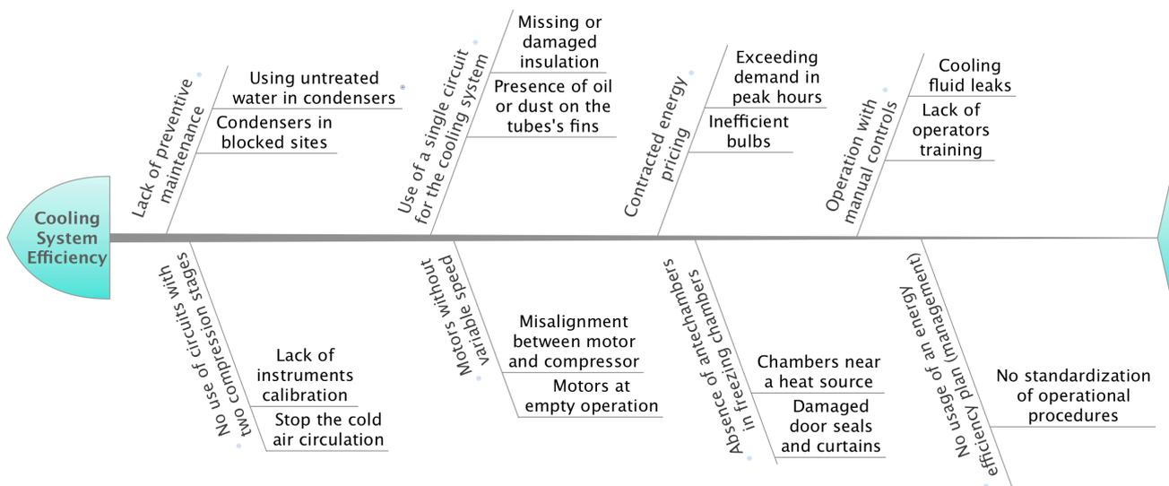
Fig. 5. Factors that lead to inefficient cooling system, in a fishbone diagram.
