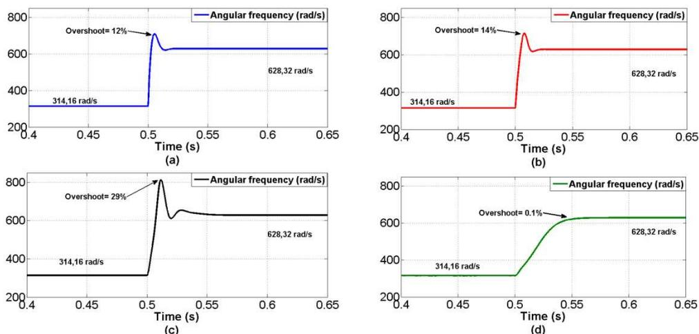
Fig. 2. Time evolution of the detected frequency when a step of frequency is exerted. a) dq PLL, b) PSD+dpPLL, c) DSOGI-PLL, d) MSOGI-FLL.
