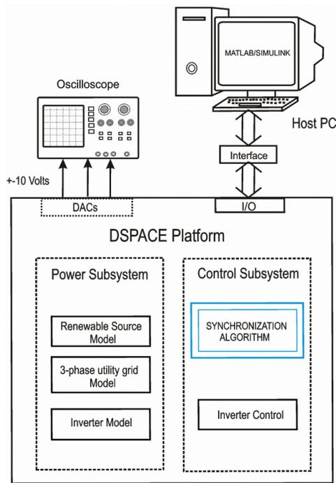
Fig. 3. Configuration of the DSPACE platform for the real time testing using a host PC, a DS1006 DSPACE board with a digital to analog converter interface and an oscilloscope for parameters monitoring.
