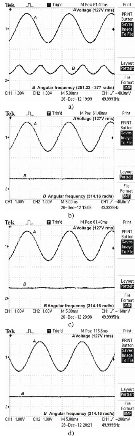
Fig. 6. Time evolution of the real-time frequency detection when voltage unbalances occurs. a) dqPLL, b) PSD+dqPLL, c) DSOGI-PLL, d) MDSOGI-FLL.
