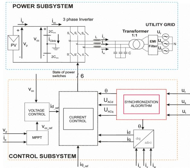
Fig. 1. Block diagram of the Power and Control Subsystems of the 3-phase PV grid-connected system used for testing the synchronization algorithms in the paper.
