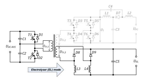
Fig. 4. Power circuit configuration in the electrolyser (EL) mode.
