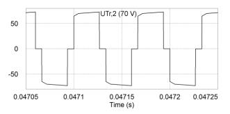
Fig. 9. General operating waveforms of the proposed multiport converter during the FC mode: secondary winding voltage of the isolation transformer  $(U_{Tr,2})$ .
