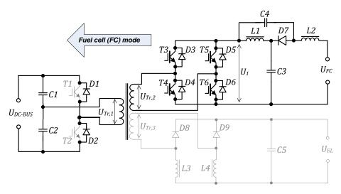
Fig. 5. Power circuit configuration in the fuel cell (FC) mode.
