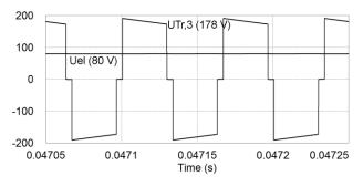
Fig. 7. General operating waveforms of the proposed multiport converter during the EL mode: electrolyser voltage ( $U_{EL}$ ) and tertiary winding voltage of the isolation transformer ( $U_{Tr,3}$ ).
