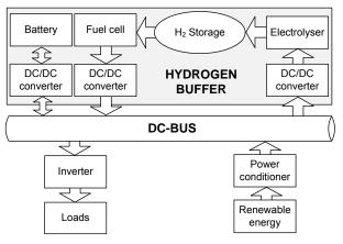
Fig. 1. Typical structure of the distributed energy system with hydrogen buffer interfaced via individual converters.
