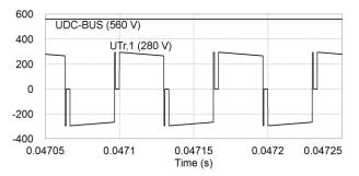
Fig. 6. General operating waveforms of the proposed multiport converter during the EL mode: DC-bus voltage ( $U_{DC-BUS}$ ) and primary winding voltage of the isolation transformer ( $U_{Tr,1}$ ).
