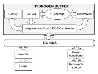
Fig. 2. Proposed structure of the distributed energy system with hydrogen buffer interfaced via multiport converter.
