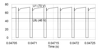
Fig. 8. General operating waveforms of the proposed multiport converter during the FC mode: fuel cell voltage  $(U_{FC})$  and intermediate DC-link voltage  $(U_I)$ .
