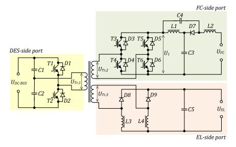
Fig. 3. Power scheme layout of the proposed integrated converter for hydrogen buffer interfacing in DES.
