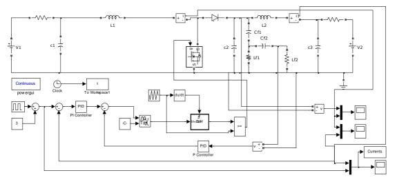
Fig.13. The PV converter current mode control block diagram
