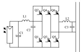
Fig.1 Single phase PV converter using a three-phase bridge
