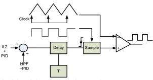
Fig.12 Sampled PWM Block Diagram IL2
