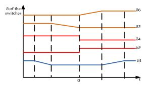
Fig.3 The PV converter switches behavior x-axis: desired voltage at the output of the H-bridge y- axis: the duty ratio of the switches to be operated.
