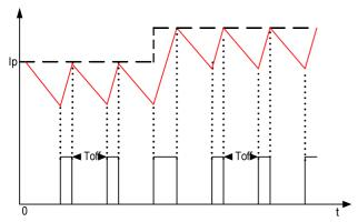
Fig. 4. Constant off Time Peak Current Control
