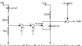
Fig.6. Constant off Time Peak Current Control Circuit with high pass filter feedback
