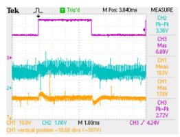
Fig.11. Constant Off time peak current control with HP feedback.
