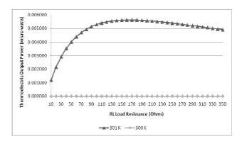
Fig. 9. The electrical power generated at the load resistor (RL) with a temperature gradient of 1 Kelvin between both sides of the device
