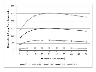
Fig. 11. The electrical power generated at the load resistor (RL) with different temperature settings applied to the thermal contact connected to Copper 1, and a doping level of 1e<sup>+</sup>16cm<sup>-3</sup> for both P-type and N-type pellets
