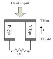
Fig. 2. A single thermoelectric couple connected for thermoelectric power generation [3]
