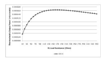
Fig. 13. The electrical power generated at the load resistor (RL) for a single thermoelectric couple with ceramic plates, and a temperature gradient of 1 Kelvin between both sides of the device
