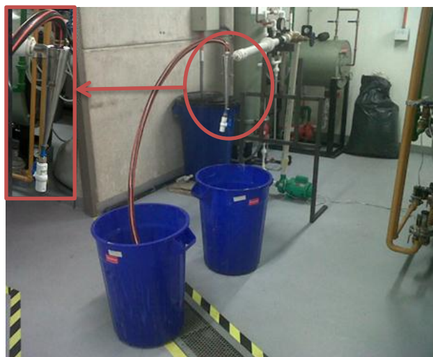
Fig.5. Hydrocyclonic system. Amplified image of the hydrocyclone (shown in the upper part at the left).
