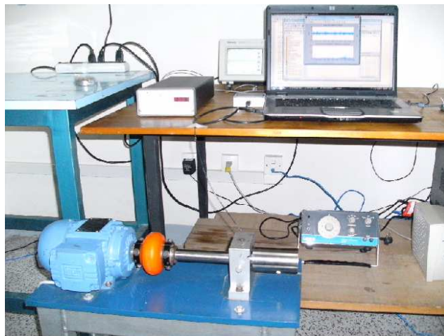
Fig. 3 – Mounting structure for bearing and related motor.
