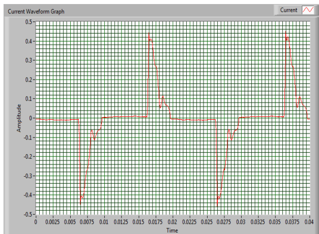
Fig. 7. Current waveform graph of ECO Energy saving light, THDI=113,12%
