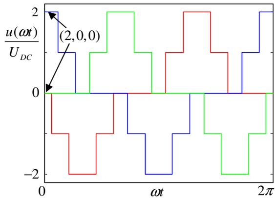
Fig. 5. Phase to ground voltages of the example given in Fig. 2
