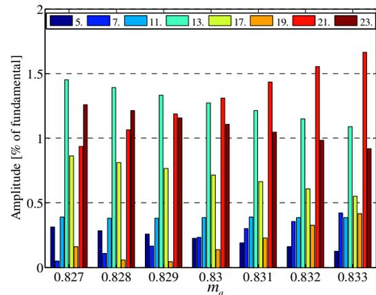
Fig. 7. Harmonics in dependence of  $m_a$  (SVFFM)
