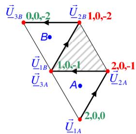
Fig. 3. Moving through the space vector diagram
