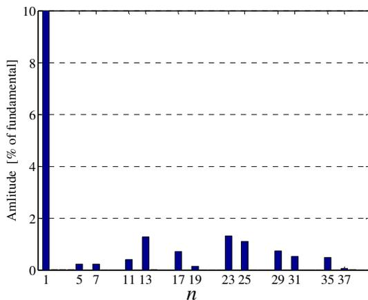
Fig. 11. Spectrum of the SVFFM for  $m_a = 0.830$
