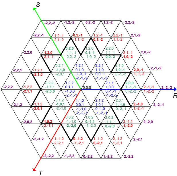
Fig. 2. Space vector diagram of a 5-level converter
