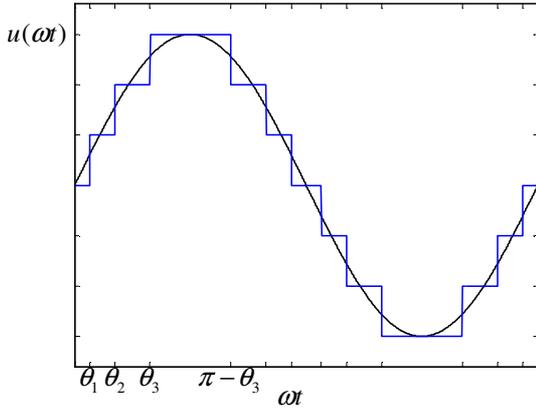
Fig. 1. Staircase voltage waveform
