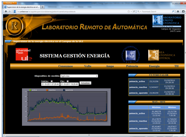
Fig. 2. Web-based monitoring system of the electrical variables at the University of León.
