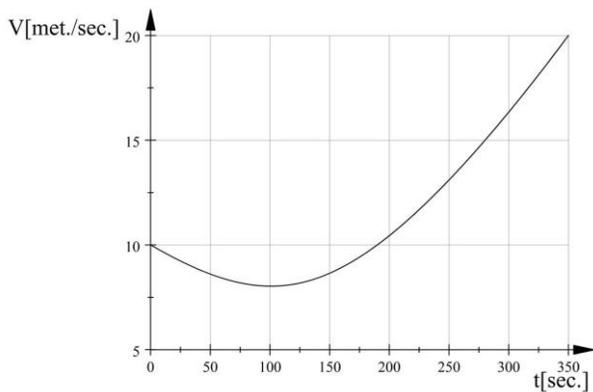
Fig. 10. Time history of the velocity  $V(t)$  in Example 2.
