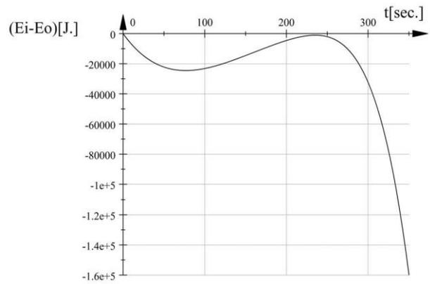
Fig. 8. Time history of the energy balance during flight in Example 1.
