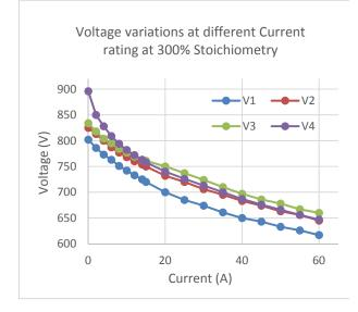
Figure 3. Cell voltage variation from OCV- 60A load for the 4 cell stack at 300% air Stoichiometry
