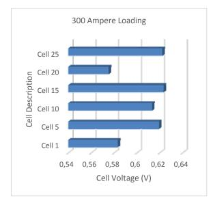
Figure 11. Ballard Mark  $9^{TM}$  cell to cell variation at 300 amps.
