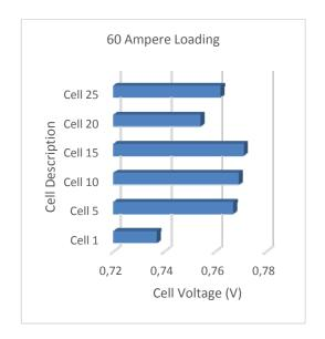
Figure 8. Ballard Mark  $9^{TM}$  cell to cell variation at 60 amps.
