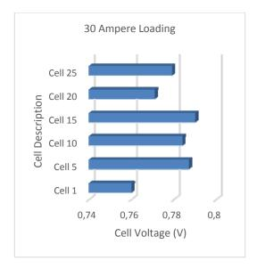
Figure 7. Ballard Mark  $9^{TM}$  cell to cell variation at 30 amps.
