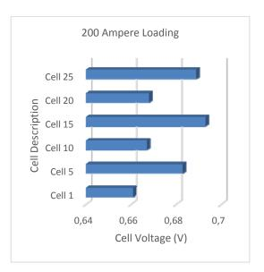
Figure 10. Ballard Mark  $9^{TM}$  cell to cell variation at 200 amps.
