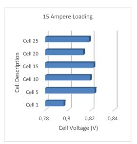
Figure 6. Ballard Mark  $9^{TM}$  cell to cell variation at 15 amps.
