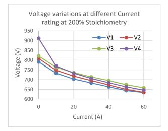
Figure 2. Cell voltage variation from OCV- 60A load for the 4 cell stack at 200% air Stoichiometry
