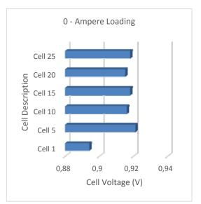
Figure 5. Ballard Mark  $9^{TM}$  cell to cell variation at OCV.
