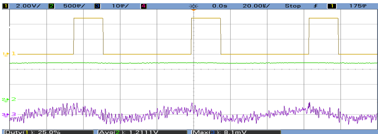
Fig.8: Ripple for a 25% Duty Cycle (12.5W) Represented on Channel 3
