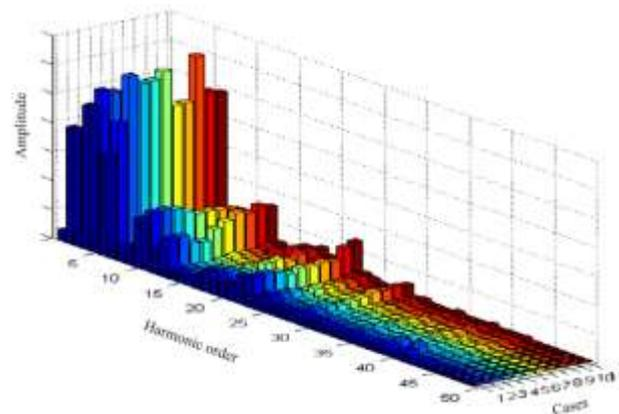
Fig 6. Current harmonics emission from wind turbine ( $\cos(\varphi) = 1$ )
