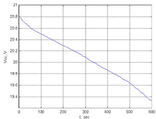
Fig. 3. The open circuit voltage decreasing, from the moment when the PV panel was exposed to the Sun, in the absence of the forced cooling air circulation.
