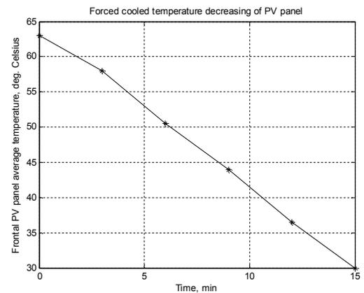
Fig. 8. PV panel average temperature decreasing, in the presence of the forced air cooling circulation, during its exposure to the Sun radiation.
