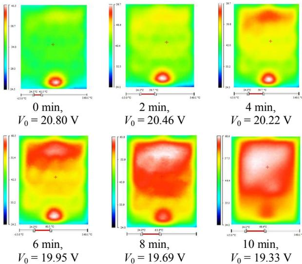
Fig. 5. The PV panel front temperature distribution, in the absence of the cooling air forced circulation.
