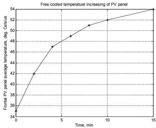
Fig. 7. PV panel average temperature increasing, in the absence of the forced air cooling, after its exposure to the Sun radiation.
