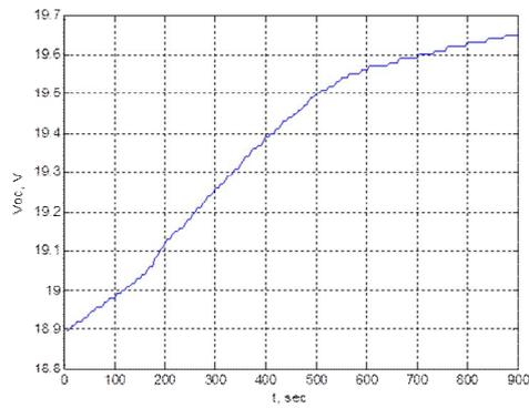
Fig. 4. The open circuit voltage increasing, in the presence of the forced cooling air circulation.
