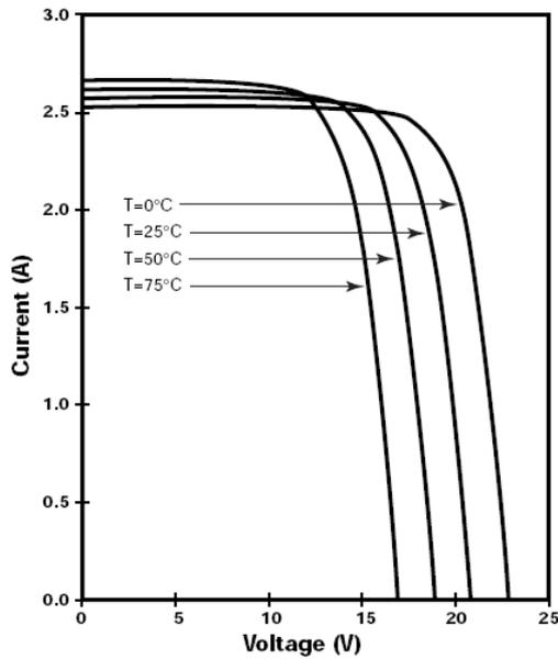
Fig. 1. The I-V curves of the investigated PV panel, for an irradiation of 1 kW/m<sup>2</sup>, at spectral distribution of AM 1.5, at various temperatures.
