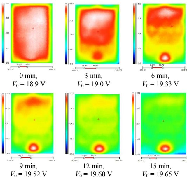
Fig. 6. The PV panel front temperature distribution, in the presence of the air cooling forced circulation; the initial value was established in the absence of the cooling air forced circulation.
