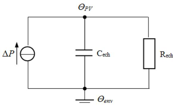
Fig. 9. Electrical equivalent circuit of the simplest thermal model of the PV panel.
