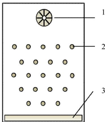
Fig. 2. The back side arrangement of the PV panel for thermal experimental investigation: 1 – a centrifugal fan, 2 – distributed air input holes, 3 – the bottom air input window.
