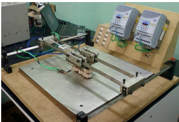
Figure 6 - Overview of the prototype built for the test of the Induction Planar Actuator
