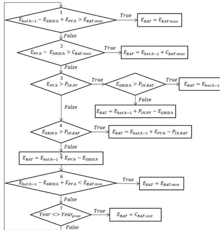
Figure 3. Algorithm for the management of PV-ESS system.
