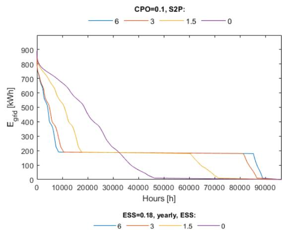
Figures 7a and b. Load duration curves with fixed CPO factor, varying three ratio between the storage capacity S2P and the peak power
