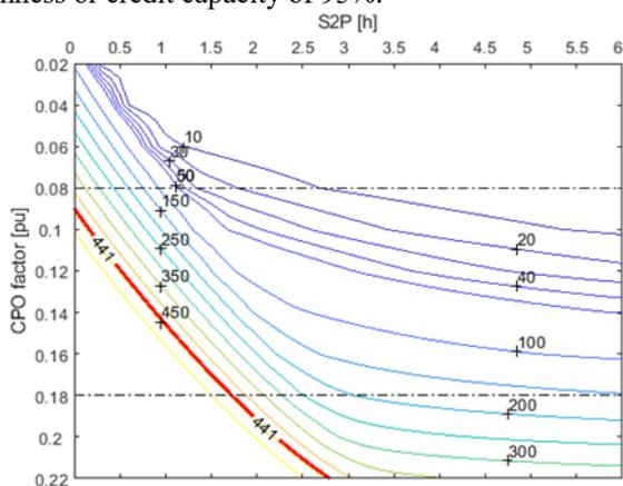
Figure 8. Annual number of hours of energy deficit with respect to the setpoint value. In red the contour curve that guarantees a capacity credit of 95%.
