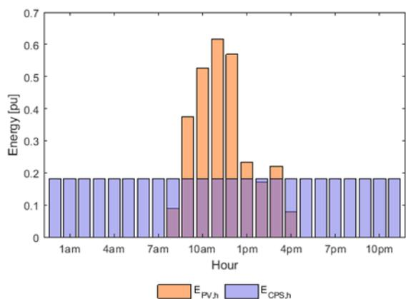
Figure 1. Constant energy setpoint (ECPS,h) and energy produced by the photovoltaic installation (EPV,h) within 1 day.
