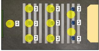
Figure 3. Diagram of the location of the light pipes and the sensors in the prototype.
