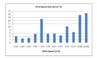
Fig. 4. Site Wind speed distribution (50m height)
