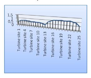
Fig. 10. Wake loss Variation for each turbine
