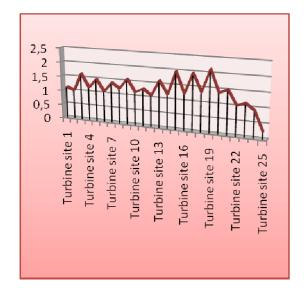
Fig. 8. Wake loss Variation for each turbine
