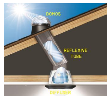
Fig. 1. - Tubular lighting system [12]
