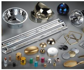
Fig. 9 – Metallic parts obtained for Vacuum Metallization [26]
