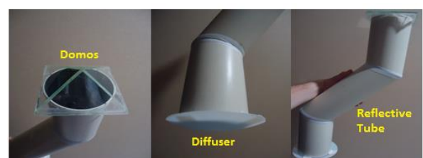
Fig. 11 – Prototype of direct sunlight lamp
