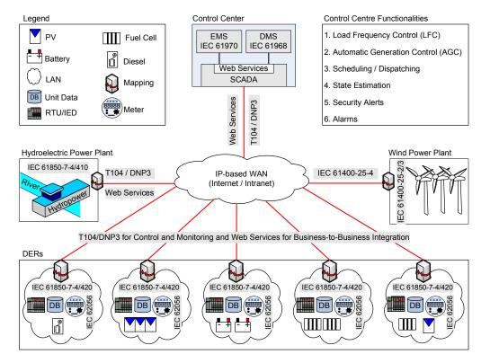
Fig. 6. Standards that can be used for the control of ECSs based on RESs and DERs over IP-based Networks.
