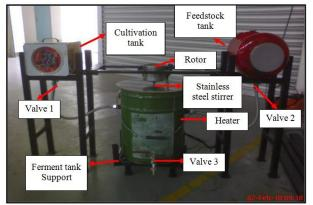
Fig. 1. Construction of a small-scale bioreactor system.
