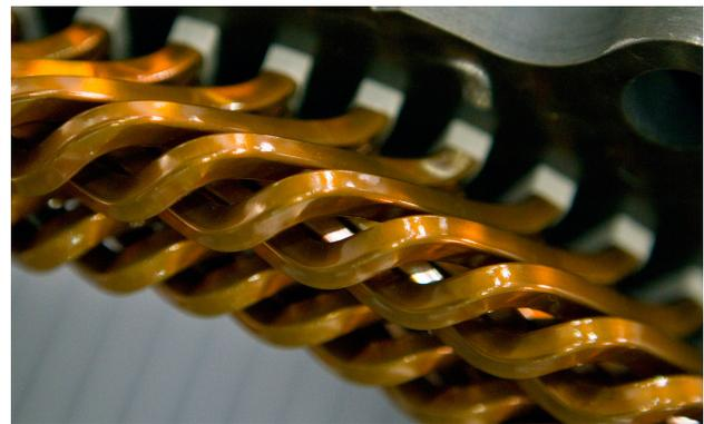
Fig. 1. Hairpin winding. Source: <http://blog.caranddriver.com/we-build-the-chevy-spark-ev%E2%80%99s-ac-permanent-magnet-motor/>.
