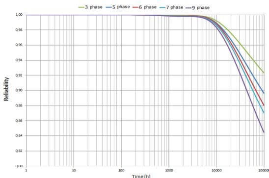
Fig.2. Reliability function R(t) of the 3,5,6,7 and 9-phases PSM
