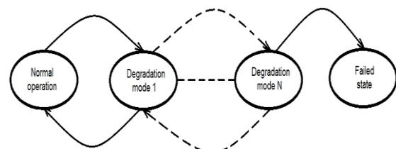
Fig.6. Multi-state Markov model of fault tolerance estimation
