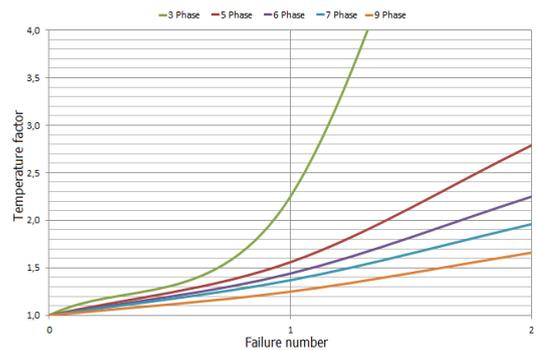
Fig.3. Overheating of stator windings in failure case (one/two phases open-circuit, 100% load)
