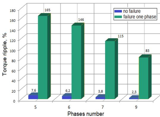
Fig.7. Electromagnetic torque ripple of PSM on the number of phases
