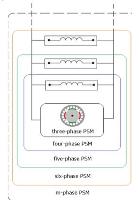
Fig.5. Structural model of multi-phase electric motor
