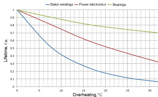
Fig.4. Overheating influence on the lifetime of the parts of electric drive
