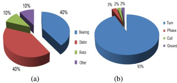
Fig.1. Statistics of the failures of PSM (a) and its stator (b)
