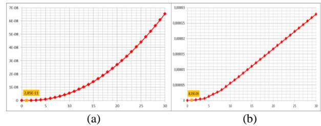
Fig.9. Probability function of complete failure of 6-phase PSM
