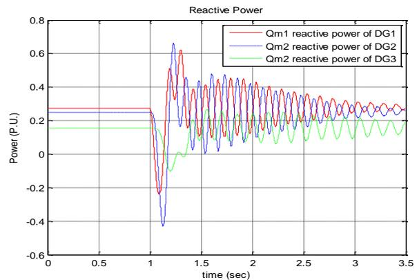
Fig. 7. Output reactive power response of the microgrids
