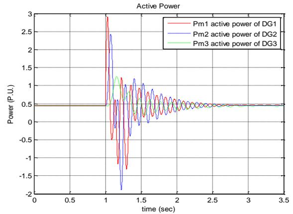
Fig. 6. Output active power response of the microgrids when the fault occurs at load1
