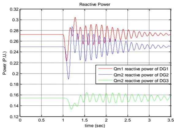
Fig. 11 Output reactive power response of the microgrids
