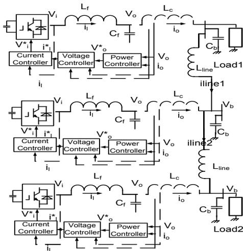
Fig. 1 Autonomous microgrid
