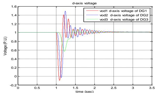
Fig. 8. Output voltage (d-axis) response of the microgrids
