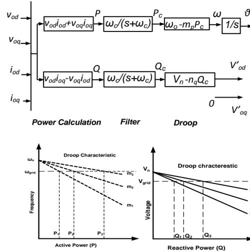
Fig. 2 Power controller and Droop characteristics
