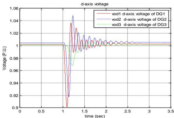
Fig. 12 D-axis output voltage response of the microgrids
