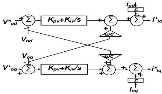
Fig. 3 Voltage controller
