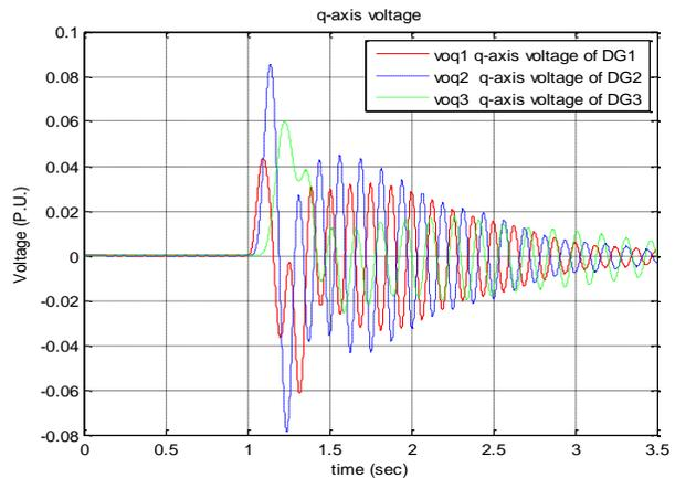
Fig. 9 Output voltage (q-axis) response of the microgrids
