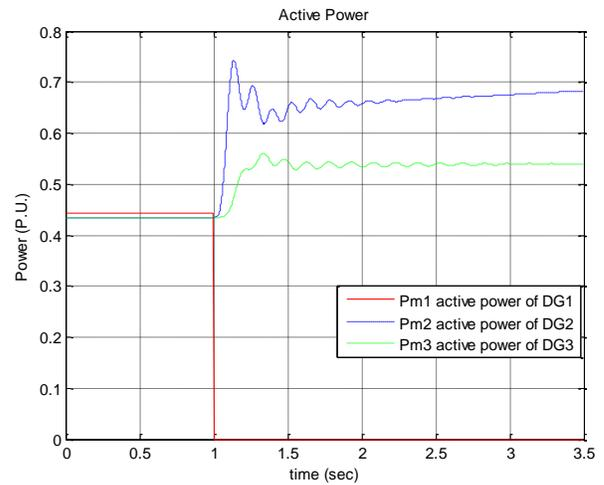
Fig. 13 Output active power response of the three DGs when the DG1 has been lost
