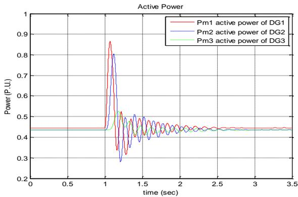
Fig. 10 Output active power response of the microgrids when the step response occurs at DG1
