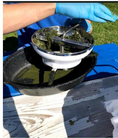
Fig. 4. Tomato processor used to make algae paste
