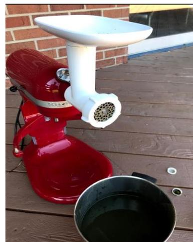
Fig. 5. Meat grinder used to create algae paste
