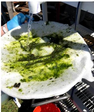
Fig. 3. Cheesecloth used to separate the algae from the water
