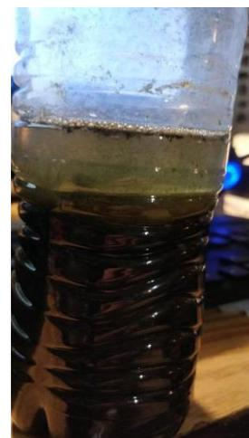
Fig. 6. Oil yield after two days of freezing and thawing
