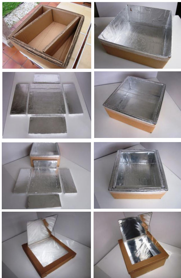
The photographic sequence shows phases of the construction process of a solar oven used as didactic model of research in bioclimatic construction.
