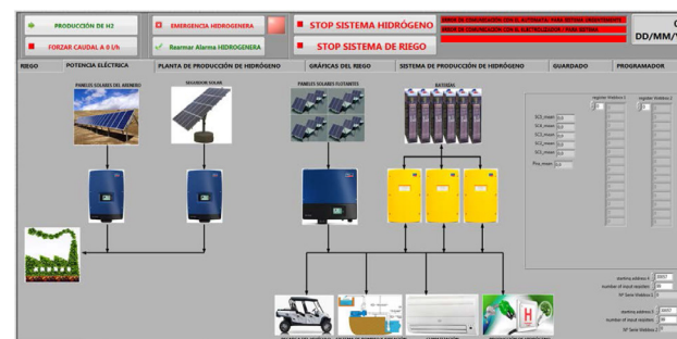
Fig. 9. Picture of the touchscreen (monitor) of the system. Detail of the two prototypes.
