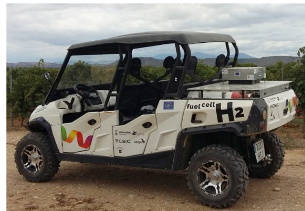
Fig. 4. View of the off-road vehicle equipped with a fuel cell.
