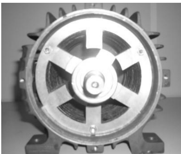
Fig. 3. Variable reluctance machine used to obtain the parameters to the simulation.
