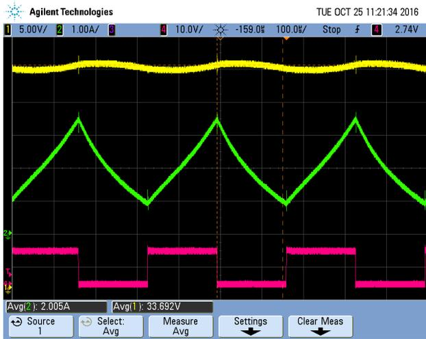
Fig. 11b. Experimental waveforms measured in the DC/DC converter with high ripple: output voltage (top), inductor current (middle), duty cycle (bottom).
