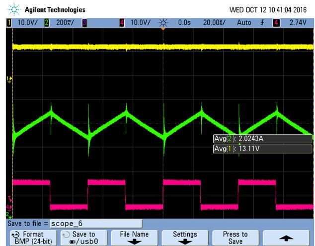
Fig. 11a. Experimental waveforms measured in the DC/DC converter with small ripple: output voltage (top), inductor current (middle), duty cycle (bottom)
