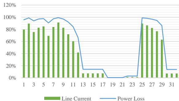
Fig. 8. Percentage of line currents and loss reduction in case 22
