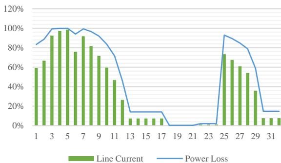
Fig. 6. Percentage of line currents and loss reduction in case 13
