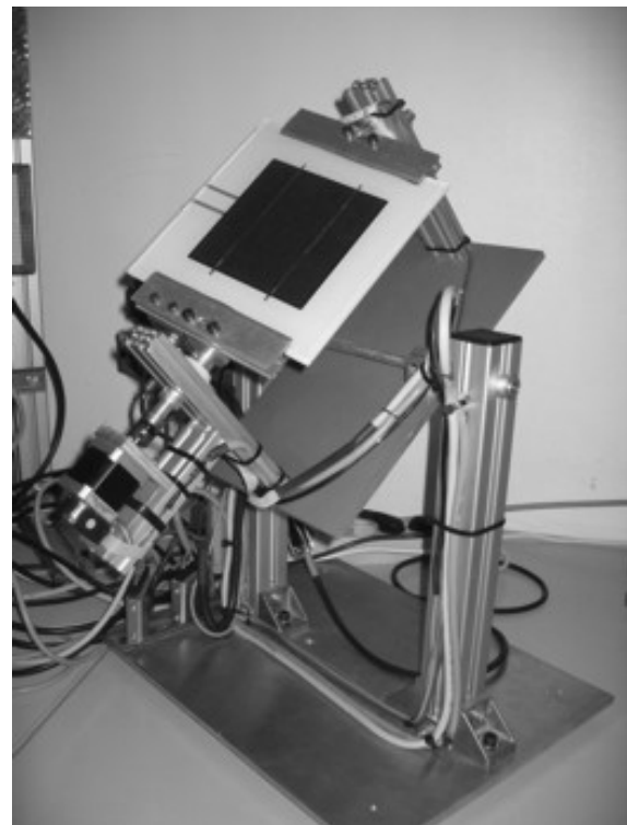
Fig. 7. Prototype built: Electromechanical structure
