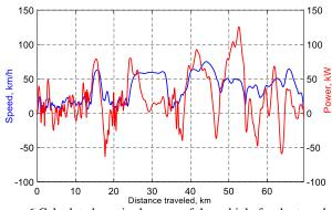
Figure 6 Calculated required power of the vehicle for the traveled route
