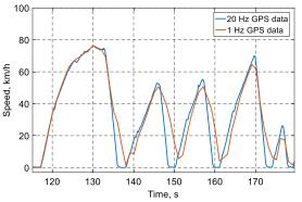
Figure 5 A comparison of speed measurements obtained with a different frequency
