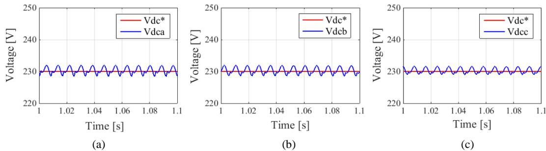
Fig. 7. DC-bus voltages of the 3FB-I-DC-Bus topology: (a) Phase “a”; (b) Phase “b”; (c) Phase “c”.
