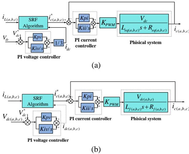
Fig. 3. Block diagrams of the current and voltage controllers: (a) 3FB-C-DC-Bus diagram; (b) 3FB-I-DC-Bus diagram.
