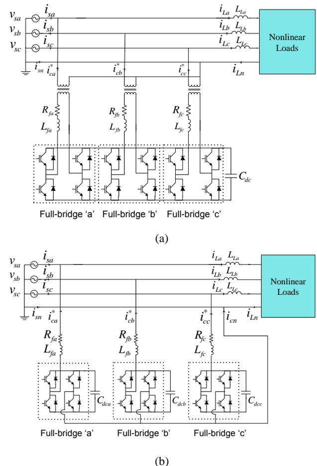
Fig. 1. SAPF Topologies: (a) 3FB-C-DC-Bus SAPF topology; (b) 3FB-I-DC-Bus SAPF topology.
