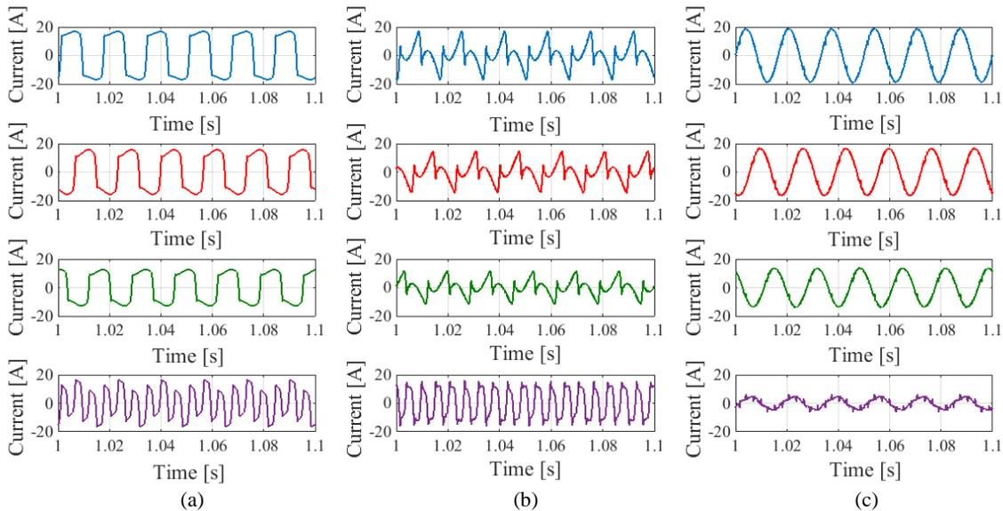
Fig. 5. 3FB-I-DC-Bus: (a) Load and neutral currents; (b) Compensation currents; (c) Grid and neutral currents.
