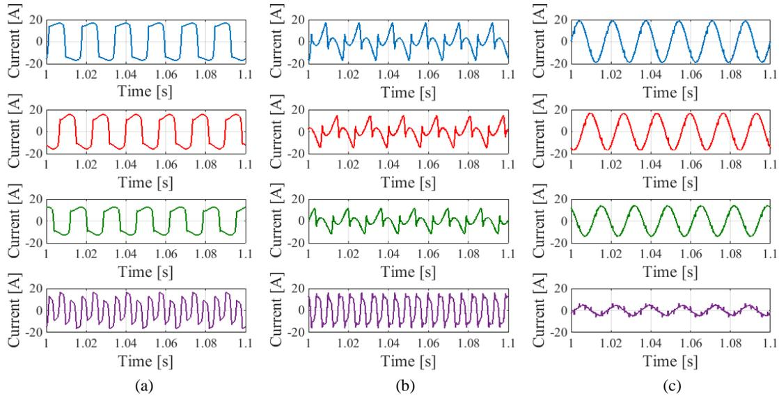
Fig. 4. 3FB-C-DC-Bus: (a) Load and neutral currents; (b) Compensation currents; (c) Grid and neutral currents.
