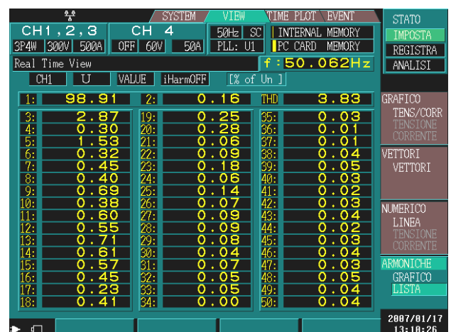
Fig. B1. Voltage harmonic values for two electronic discharge lamps
