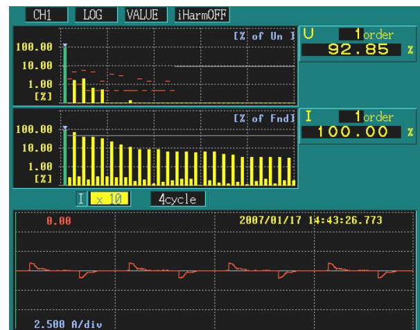
Fig. 3. Current waveform and voltage and current spectra for two electronic discharge lamps
