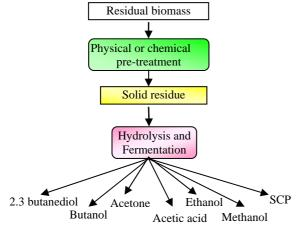
Figure 2. - Obtaining of different products from lignocellulosic residues
