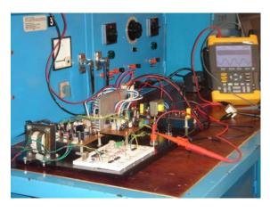
Fig. 16. Power stage of the full bridge inverter.
