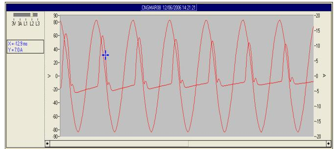
Fig. 3: Field data, voltage and current transient
