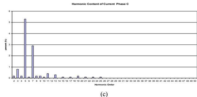
Fig. 6: Individual harmonics for line currents
