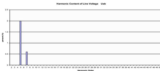
Fig. 5: Individual harmonics for Uab line voltage
