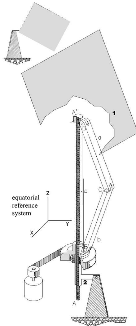
Fig.5. Mechanic scheme of the heliostatic illuminator
