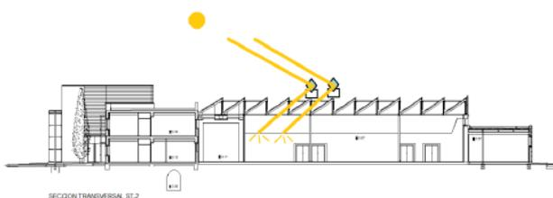
Fig.4. Installation scheme of heliostats as a daylighting element for the classrooms of the Leonardo da Vinci building of the Campus of Rabanales at the University of Córdoba (Spain).
