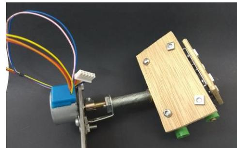
Fig.9. 1:15 Scale model of the single axis polar heliostats
