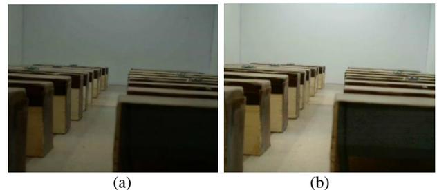
Fig. 16. Qualitative comparative analysis of daylighting levels inside the scale model without heliostat illuminators (a) and the one with heliostat illuminators (b).
