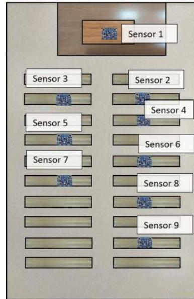
Fig.8. Layout of the TSL2561 sensors inside the 1:15 scale model of the chosen classroom of the Leonardo da Vinci building of the Campus of Rabanales at the University of Córdoba (Spain).
