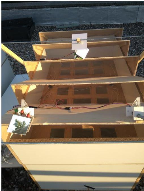
Fig. 11. Layout of the 1:15 scale models of the heliostatic illuminators on the roof of the chosen classroom of the Leonardo da Vinci building of the Campus of Rabanales at the University of Córdoba (Spain).
