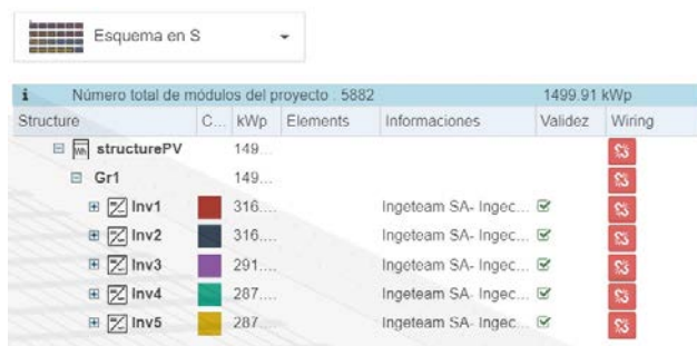
Figure 11. Electrical connections among solar modules in S shape and the number of inverters planned.
