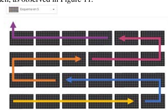
Figure 10. S disposition to connect solar panels.
