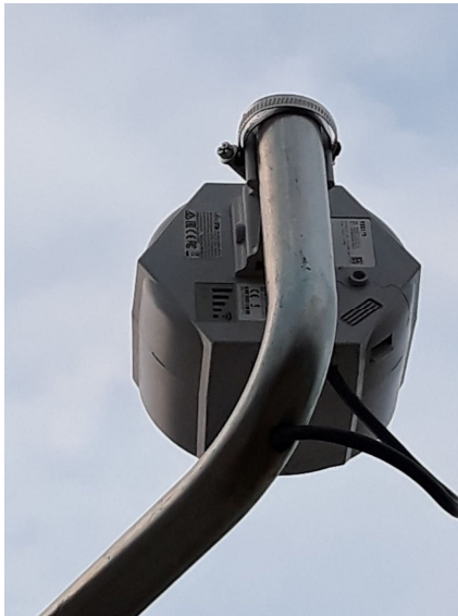
Fig.9: 10-dbi directive Mikrotik antenna to increase the 4G signal level. I+D Energías, Poland
