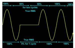
Figure 3. Example of another problem solved by IEC 61000-4-30. Is this dip 50% for two cycles, or 0% for 1 cycle? Again, <u>both answers are technically correct</u>. 61000-4-30 makes it clear that this is a dip to 0% for 1 cycle – thus reducing cost of instrumentation.
