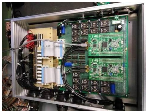
Fig. 16. Real controller with ARM CORTEX M4 microprocessors
