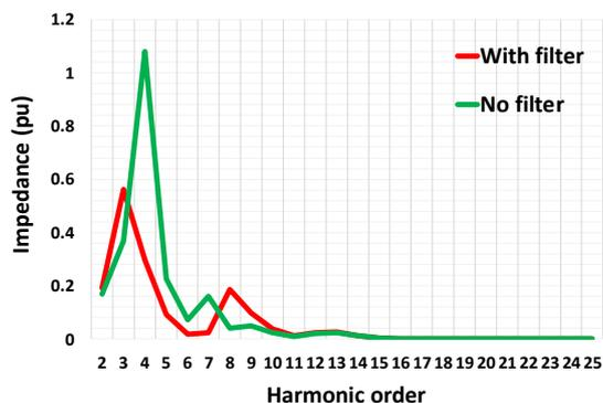
Fig. 7. Impedance-frequency response before and after connecting the 7<sup>th</sup> order tuned filter.
