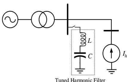
Fig. 1. Representation of a grid-connected tuned harmonic filter.
