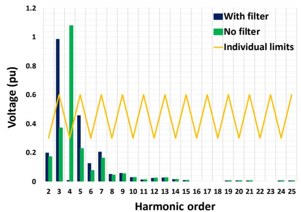
Fig. 4. Voltage harmonic spectrum before and after connecting the 4<sup>th</sup> order tuned filter.
