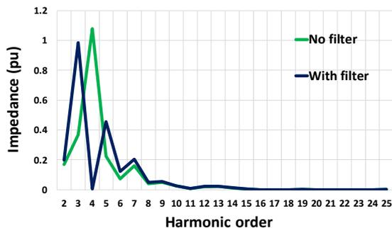
Fig. 5. Impedance-frequency response before and after connecting the 4<sup>th</sup> order tuned filter.
