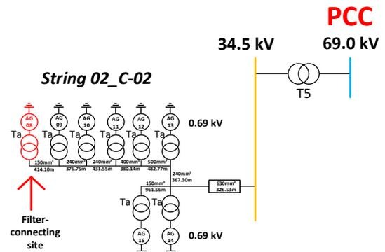
Fig. 3. Filter connecting busbar (String 02\_Circuit-02).
