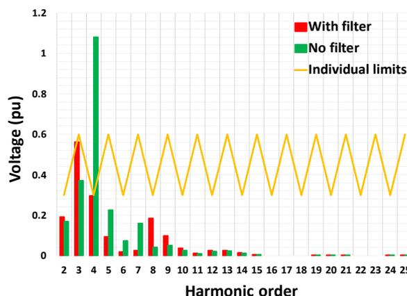
Fig. 6. Voltage harmonic spectrum before and after connecting the 7<sup>th</sup> order tuned filter.
