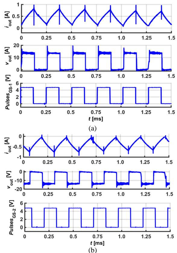
Fig. 12. Motor current, voltage and MOSFET gate-source pulses for (a) forward mode and (b) reverse mode.
