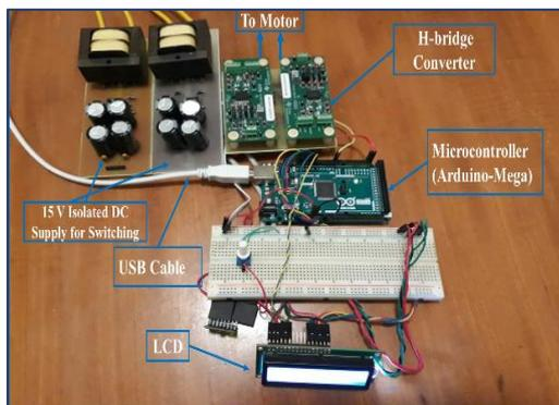
Fig. 10. Experimental setup for a four-quadrant DC-chopper
