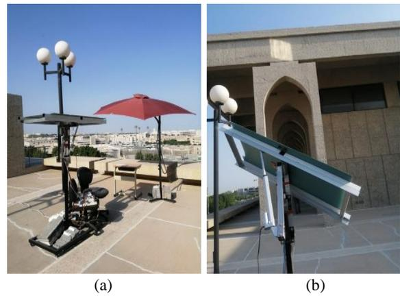
Fig. 11. The proposed prototype of the automatic dual-axis solar tracking unit.
