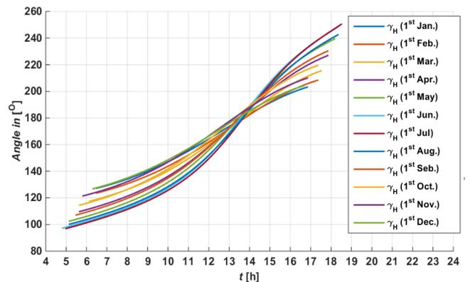
Fig. 8. Heliostat angle curves with respect to Dhahran time, the Heliostat azimuth angle,  $\gamma_H$ , from Eq. (6)
