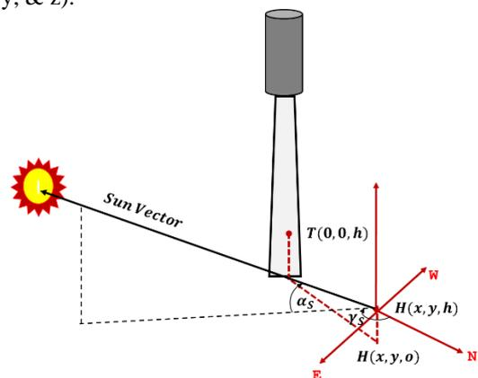
Fig. 2. Elevation and azimuth sun angles
