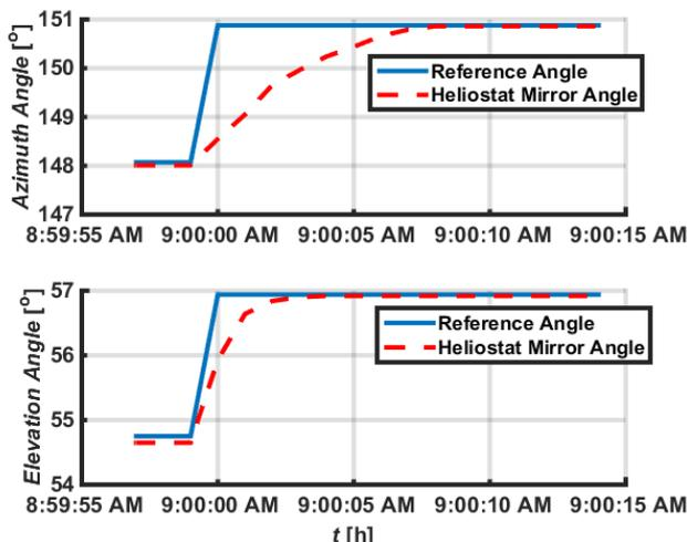
Fig. 14. Reference tracking angles for azimuth and elevation with Heliostats mirror angles at 09:00 AM
