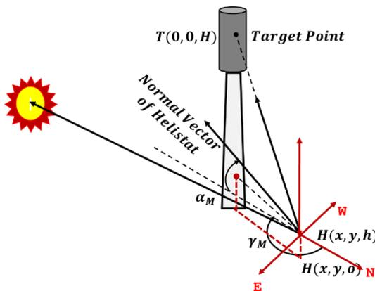
Fig. 4. Elevation and azimuth Heliostat angles
