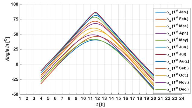
Fig. 5. Solar angle curves with respect to Dhahran time, the solar altitude angle,  $\alpha_s$ , from Eq. (2)
