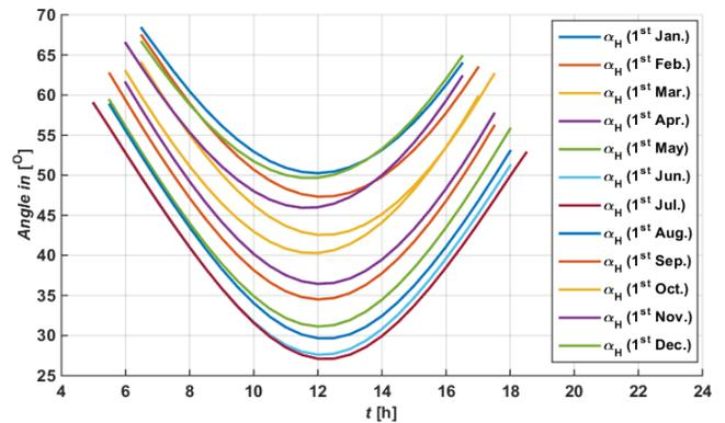
Fig. 7. Heliostat angle curves with respect to Dhahran time, the Heliostat altitude angle,  $\alpha_H$ , from Eq. (6)
