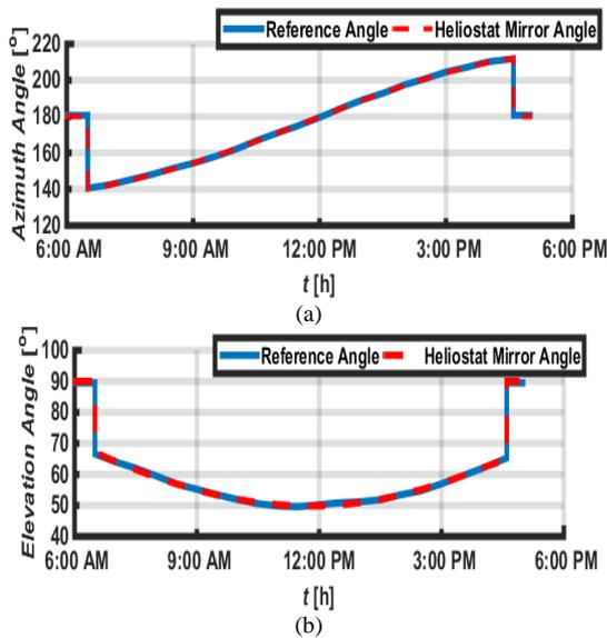
Fig. 13. (a) Reference and tracking angle for azimuth motion angle. (b) Reference and tracking angle for elevation motion angle with Heliostats mirror angles on 10<sup>th</sup>. Sep. 2019
