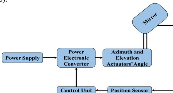
Fig. 1: Schematic diagram for the basic solar tracking system
