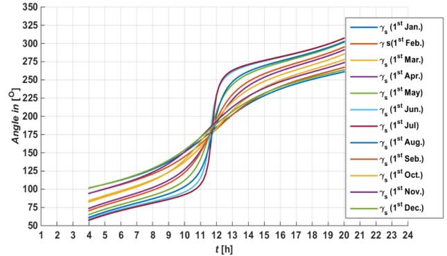
Fig. 6. Solar angle curves with respect to Dhahran time, the solar azimuth angle,  $\gamma_s$ , from Eq. (2)
