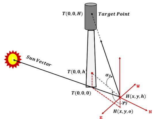
Fig. 3. Elevation and azimuth target angles
