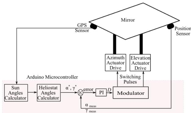
Fig. 9. Block diagram of dual-axis solar tracking system
