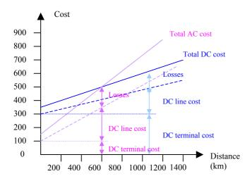
Fig. 3. HVAC-HVDC cost
