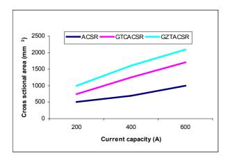
Fig. 1. Current capacity in function of the cross sectional area
