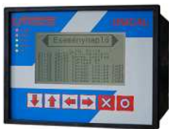
Fig. 5. UNICAL – The new intelligent data acquisition device for energy-flow measurements
