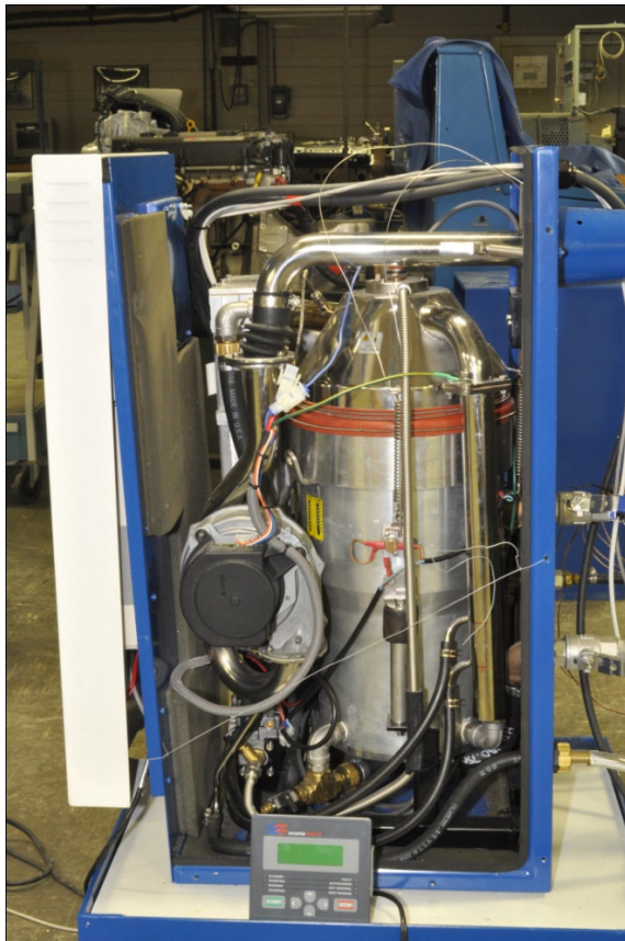
Fig. 1. The installed WhisperGen Stirling engine.
